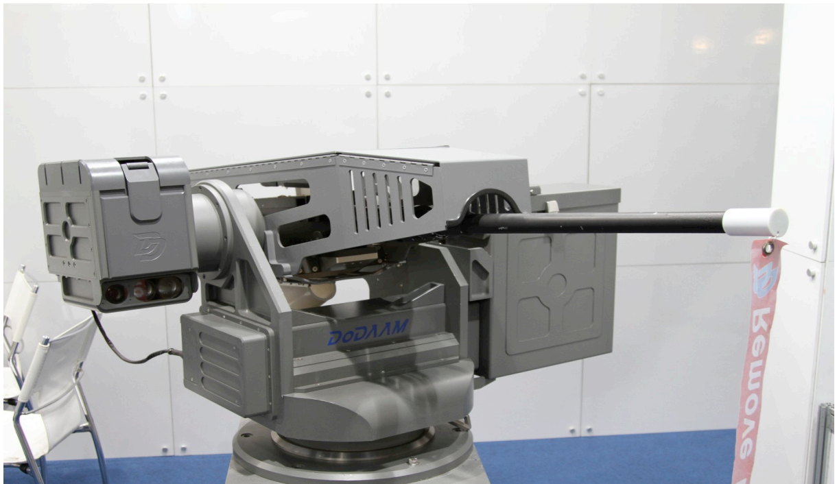
Picture 1. DoDAMM's Super aEgisII: South Korea's autonomous robot gun turret. Source: Loz Blain, 2016.
