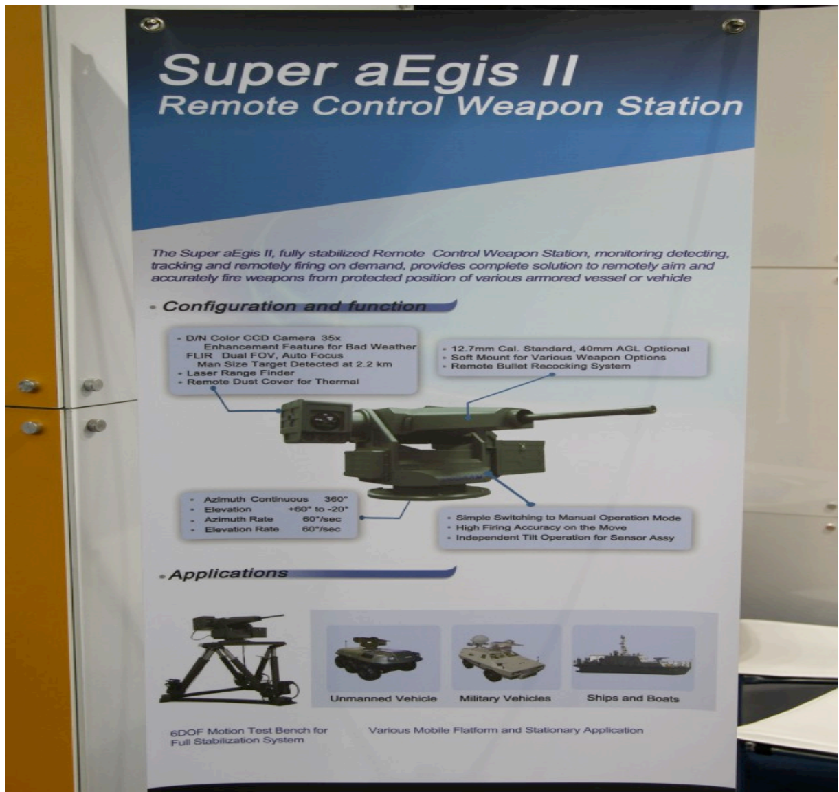
Picture 2. DoDAMM's Super aEgis II: South Korea's autonomous robot gun turret. Source: Loz Blain, 2016.
